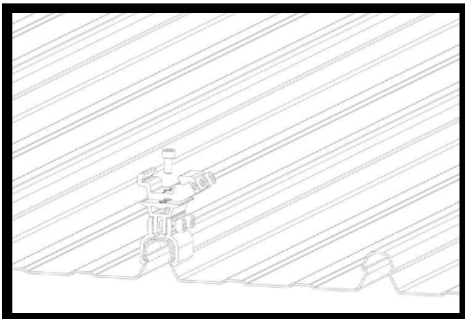
3. For flush and fixed tilts, once the Kliplok is secured on the roof sheet, mount the channel feet on top with a bolt.
