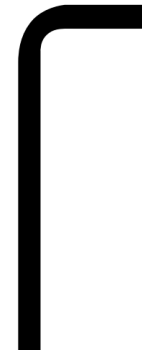
Hex Key (A 6mm hex key / driver bit is required to secure the SunLock channel to the channel feet)
